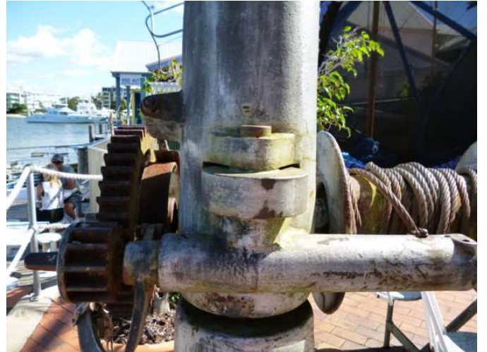
The friction brake mechanism is simple.
