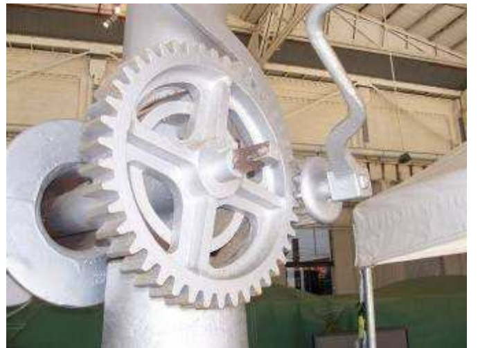
The crank handle could be located at several positions.
