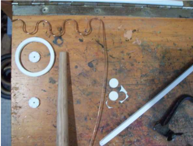
The Whip wheel spokes are curved copper wire.
